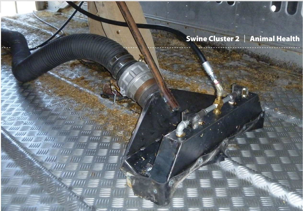
Second pass with the wet attachment to perform a pressure wash combined with vacuuming. Source: PAMI
