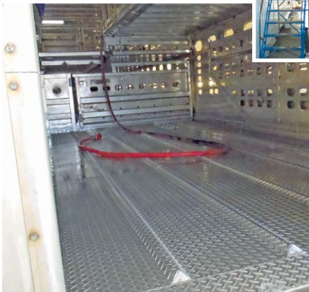
Condition of floor after flood wash. Source: PAMI
