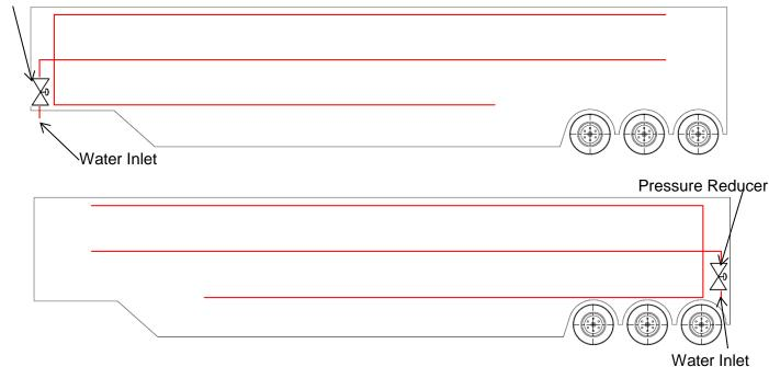
Figure 4 Possible layouts for water line configuration on one side and along the centreline of the trailer
